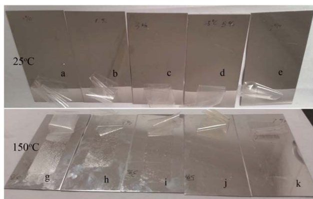
Figure 10. Thermoresistance of PSA was tested at 150 and 25°C. (a)–(e) PSA tapes were crosslinked by 0, 1, 3, 5, 7 wt % heat-resistance monomer, respectively at 25°C; (g)–(k) PSA tapes were crosslinked by 0, 1, 3, 5, 7 wt % heat-resistance monomer, respectively at 150°C (monomer ratio: BA:VAc:AA = 81:15:4 wt %; reaction temperature: 80°C; reaction time: 8 h; heating rate: 10°C/min; repeated test: three times. Peeling speed: 300 mm/min). [Color figure can be viewed in the online issue, which is available at wileyonlinelibrary.com .]
